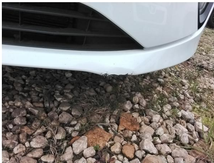
2: Bumper Front Dented With Paint Damage
