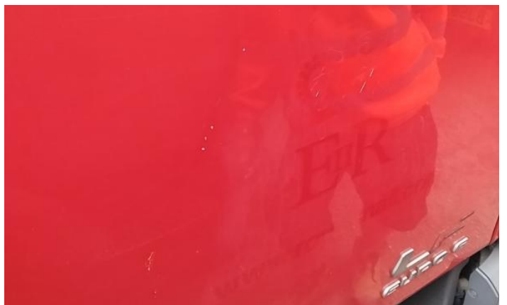
6: Door osf Scratched Over 25mm Thru Paint
