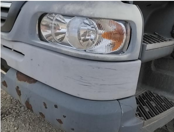
5: Bumper Front Moulding Scuffed (Unpainted) Over 100mm
