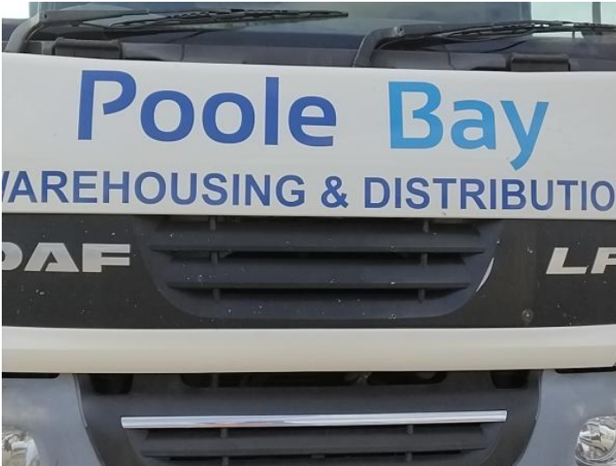
3: Grille Front Scratched (Painted) UpTo 25mm Thru Paint
