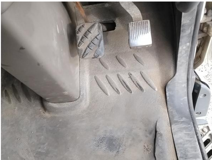
22: Carpets Front Torn Over 10mm
