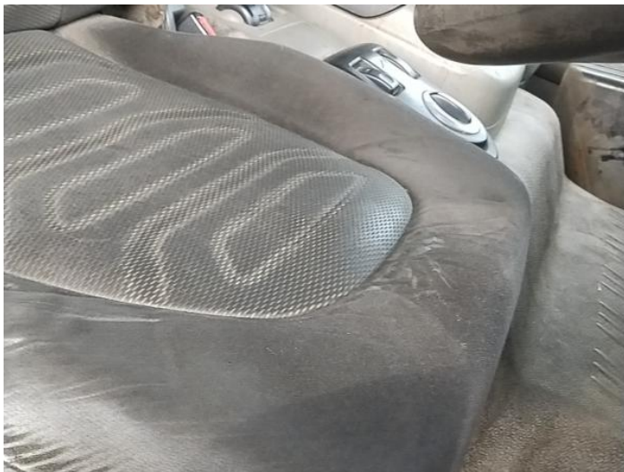
21: Seat Base Cover osf Burn Over 3mm
