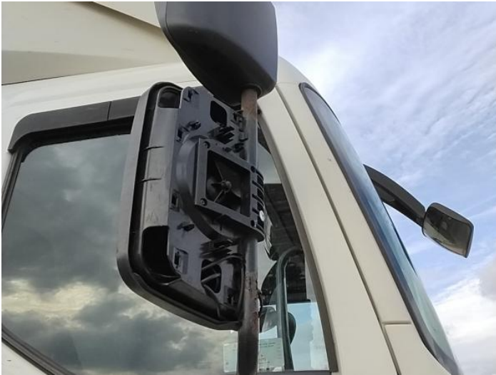
15: Door Mirror Assy osf Missing Replace
